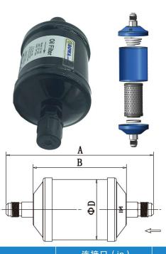
Oil filter can filtrate 99% of 3 micron grain but still have enough flow rate to maintain the low pressure drop. Oil filter has a very high capacity of filtration. It can return the cleanness POE oil and mineral oil back to the compressor. The clean oil not only can make sure the oil regulator working properly but also can reduce the abrasion of the compressor. Oil filter actually can release changing oil for compressor that caused by suspend feculence during
